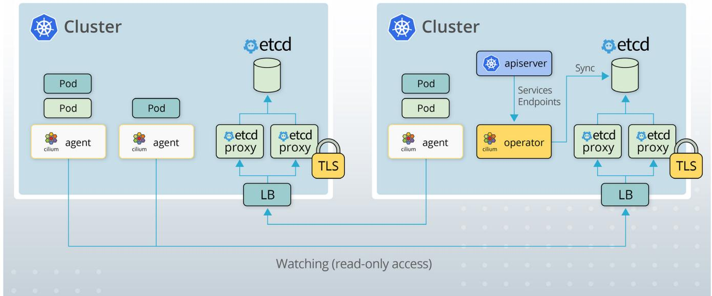
Clusters are connected and routed through VPCs using either the standard API from any cloud provider or an on-premise infrastructure via regular IPSec-based VPN gateways and tunnels or directly through network headers or via hybrid routing mode.
